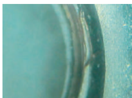
有毛邊 Burr with conventional forming tap
