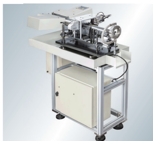
⑭ Off-line gauging, non-contact O.D. measuring system
