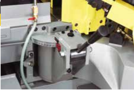
Strong Angle Cutting (R60°) by Manual 強力手動鋸弓轉角度 (正 60°)
