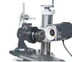
Sharpening face milling cutter being held in the C2SF fixture with a AA20-AA26 arbor, cutter is indexed with C2R1 univ tooth rest, and wheel is diamond cup wheel
