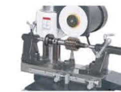
Sharpening gear hob held on C2T12 fixture with a AB01-AB04 arbor, C2R2 plain tooth rest is indexed against index disc
