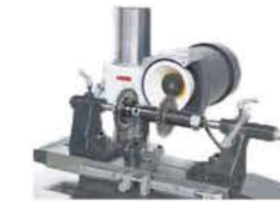
Sharpening side milling cutter held on C2T12 fixture with a AB01-AB04 arbor, C2R2 plain tooth rest is indexed against index disc
