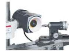
Sharpening a ball radius end mill held on C1RG attachment
