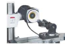
Sharpening turning tool set-up on C2LH fixture
