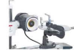
Sharpening circular saw blade held on C1SG attachment
