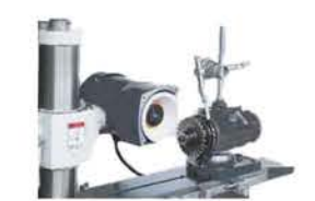
Sharpening side milling cutter held on C2SH fixture with a AA01-AA15 arbor, C2R1 plain tooth rest is indexed against index disc
