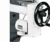
4. Power rapid up/down system
