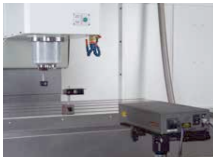
Laser inspection is applied for every machine ensure perfect quality. 雷射進行定位校準，確保最佳品質。
