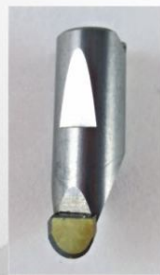
鏡片精車MCD車刀 (R2,R5)
