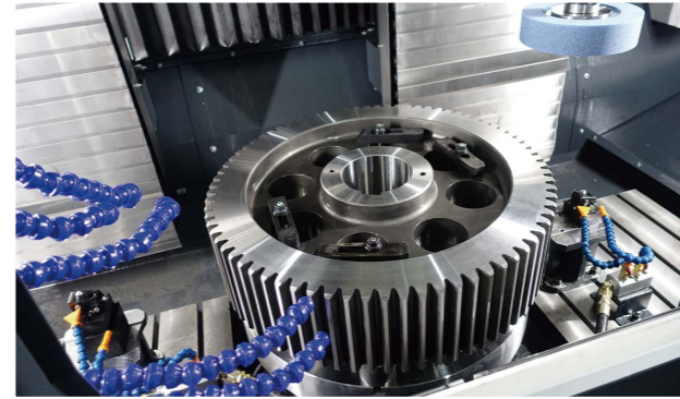
齒輪內外徑端面研磨 Gear ID, OD and flat grinding
