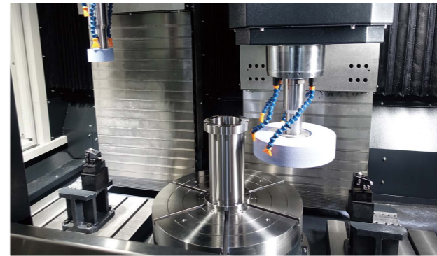
內藏主軸套管研磨 Built-in spindle grinding
