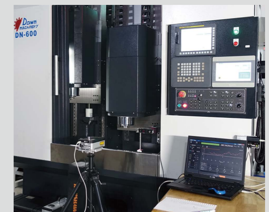
定位精度雷射檢驗 Position error measurement
