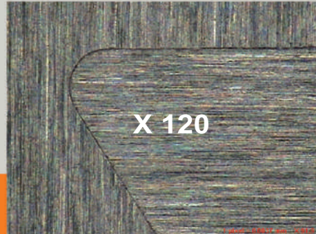
30° interior / exterior corner control Wire diameter 0.2mm
