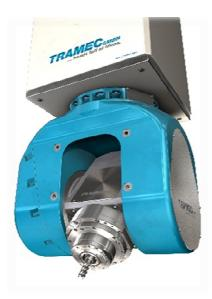
Pure high-tech. Low weight, structural rigidity and universal applicability in the machining of medium and large components. The AC 7M is more flexible due to the use of spindles up to 230 mm and the HSK-A100 tool holder.
