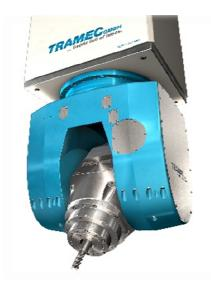
The AC 15 is designed for use iin processing light- to medium weight parts. A universal, powerful milling head for high-performance machining with great shock-absorbing properties.
