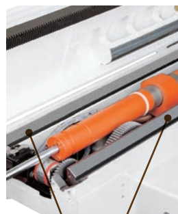
Longitudinal double "V" guideways
