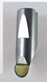
Glasses lens finishing MCD turning tool (R2, R5)
