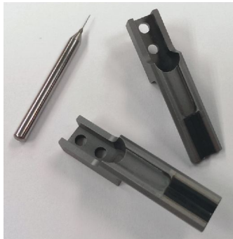
Wear-resistant workpiece for micro drill machining
