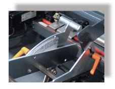
Bar diameter selection on the magazine tray is performed by a simple manual adjustment via changeover gauge, no tool required. A five position scale allows to visually seeing where the new adjustment is aligned for accuracy and quick selection.
