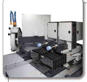
Y axis applys to sleeve type rigid grinding spindle with Ø405mm grinding wheel (wheel angle 25°) Z axis applys to BELT type grinding spindle Z2 axis applys to BELT type grinding spindle
