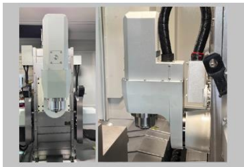
BBT30 milling spindle 24,000rpm (B axis with Harmonic gear, swivel angle \pm 105^\circ )
