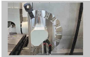
11T servo turret with Harmonic gear (right)
