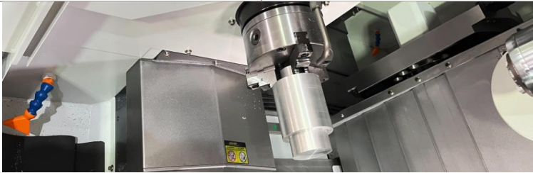
Chip flushing system (left side)
