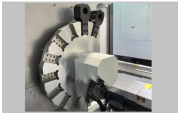
11T servo turret with Harmonic gear (left)
