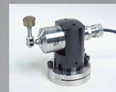
Automatic tool length measuring device (Dah Lih, Renishaw or Blum)
