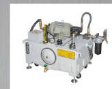
Coolant through spindle device (20,30,50,70 kgs)
