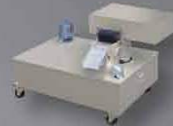
Cooling System with Magnetic Separator
