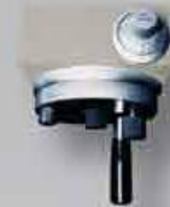
Cross Micrometer Attachment (PSGS) 1 division on cross handwheel: 0.002mm 1 revolution on cross handwheel: 0.04mm
