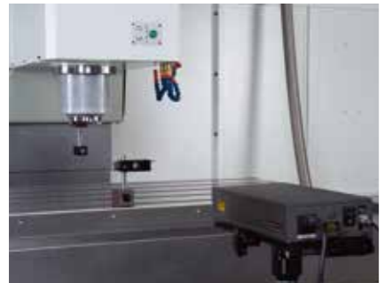
/ Laser inspection is applied for every machine after installation to ensure perfect quality. • 每座機台均以雷射進行定位校準，確保最佳品質。
