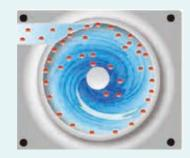
times to clean the tank, in turn minimizing the operating costs. It helps to improve machining accuracy and prevent damage to the machining surface of equipment. The cyclone effect eliminates the need to replace filter core; i.e., no consumable material needed. No bubbles are formed as it does not blend in air.
