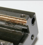
Inspection interval 3: Lubricant residue
