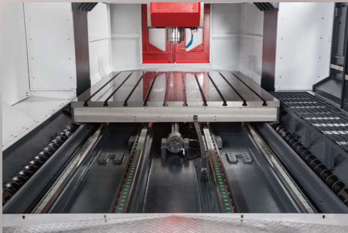
X axis with 4 linear way, High resolution ENCODER , Coolant Through Ballscrew Design.
