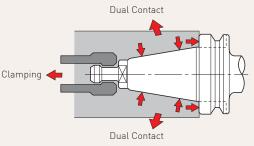
Taper Dual Contact Spindle
