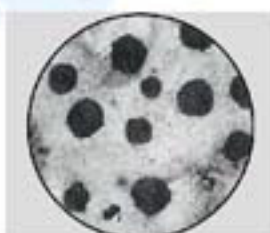
Microphotograph for ductile cast iron
