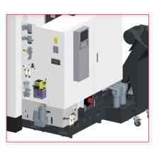
Simplified pneumatic, hydraulic, lubrication and CTS filter system easy for maintenance.
