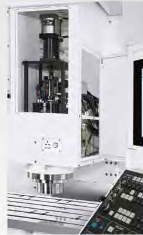
Headstock service door to facilitate access is standard on all models.
