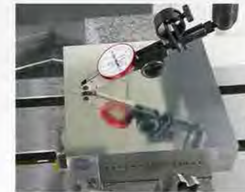
DYPEC ® mirror milling with ball end mill
