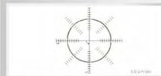
E.g. XY Double Ball Bar Test Results under 5 microns.
