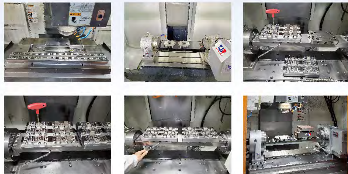
The illustration of the application for the zero point clamping system on the faceplate of the 4 th & 5 th axes
