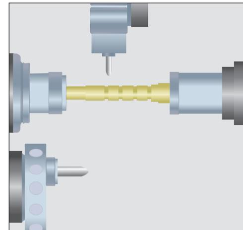
Turret 1 OD Turning & Sub-turret Back Machining
