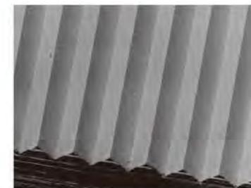
Molding of LCD display optical waveguide
