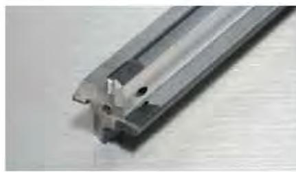
**■Finishing of Intake and Exhaust Valve Guide Holes**
