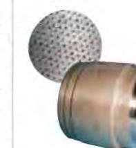
A rotary dresser with diamond grits arranged regularly made by the reverse plating method. Concentration of the diamond can be controlled according to requirements. The SZ Type provides efficient plunge dressing of large size rotary dressers.
