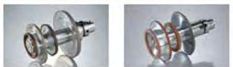
A.L.M.T.'s various flute grinding wheels mounted on arbors of tool grinders enable highly efficient and highly precise grinding regardless of grinding fluids and workpiece materials.
