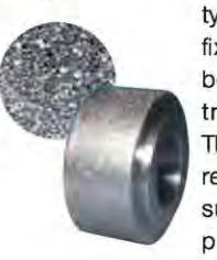
The diamond grits of Z type rotary dresser are fixed on the precise body by use of electro-plating process. This type can be made relatively easily and is suitable for small lot production and trial production.
