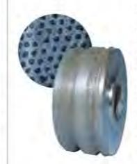
SX type rotary dresser is produced by integration of our prominent technologies the original arrangement design of diamonds, the precise sintering technology and the excellent truing technology. Therefore SX type has a high valuation in grinding applications that require sharpness. It can also be effective in traverse dressing and contour dressing.
