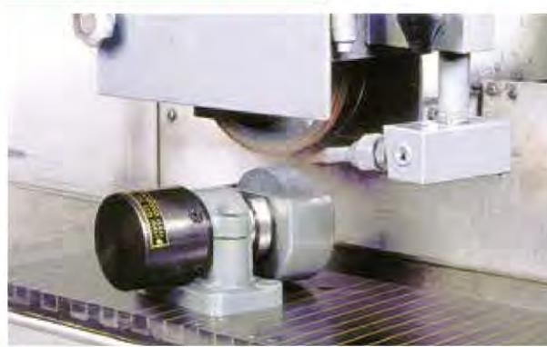
The brake dresser removes run-out with pressing force between dresser and diamond wheel as well as peripheral speed difference
