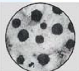
Microphotograph for ductile cast iron
