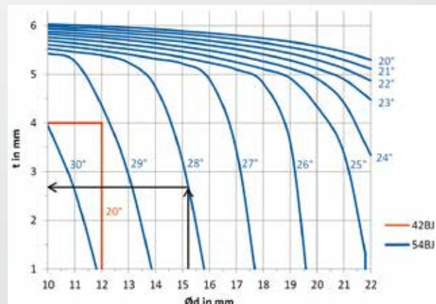
例如 54BJ:  $\Phi d = 15.2$  mm;  $\alpha = 28^\circ \rightarrow t \leq 2.7$  mm
