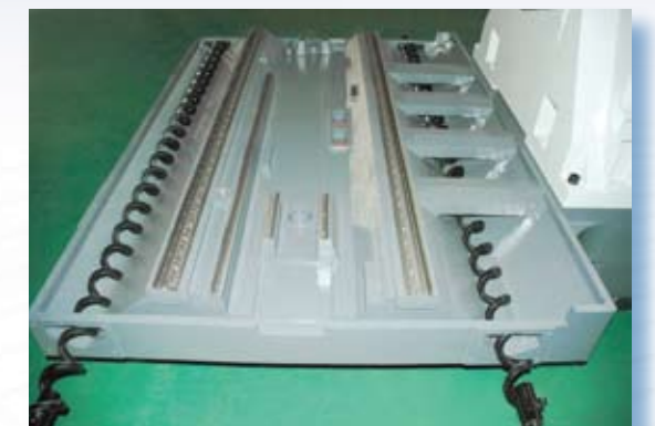
Broad base construction, dual type chip screw
