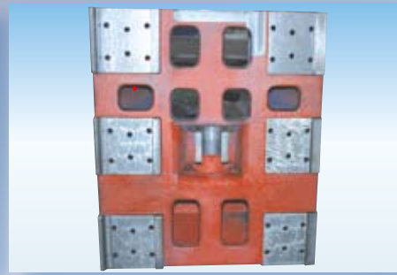
6 sliding blocks on spindle head
