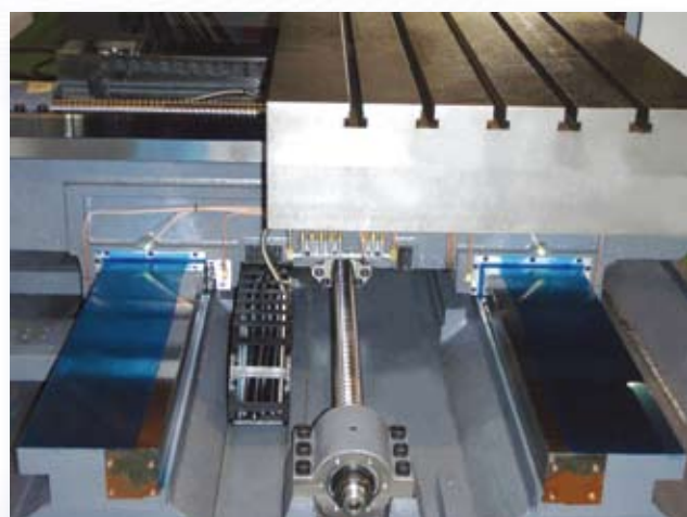
The rolling wheel of elastic cover does not damage the sliding trace
