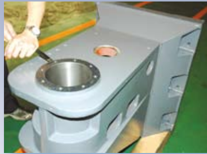
Precise head scraping for spindle
