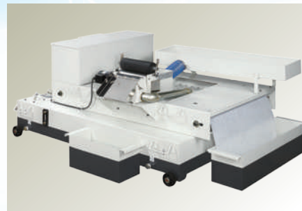
Coolant System With Auto. Paper Feeding Device & Magnetic Separator (with 1 Roll of Paper) Volume: 120L Paper feeding motor: 25W Pump: 1/8HP Coolant Capacity: 20L/min. Space: 1,450 x 620mm Height: 760mm
