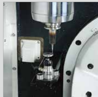
/ TOOL LENGTH MEASUREMENT DEVICE
