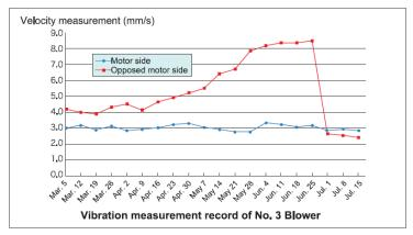
**Similarity comparison**: This method compares vibration values of machines of the same type and judges a machine of the higher vibration value (indication the machine is abnormal). **Absolute value evaluation**: This method judges the vibration value according to reference vibration values defined by machine scales by ISO 10816-1.
