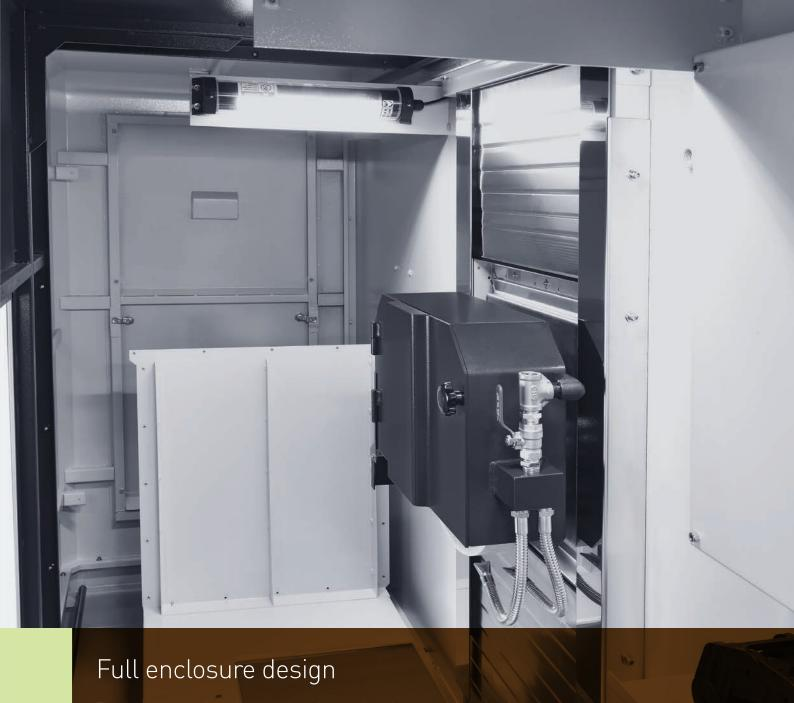
The fully enclosed design meets safety and environmental regulations by preventing cutting coolant splashing and oil mist dissipation while fully protecting the operator from grinding dangers.
