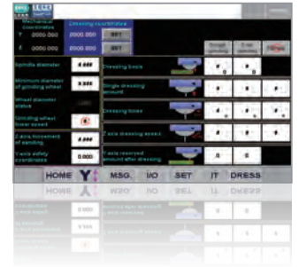
Auto wheel dressing ADC setting screen (OPT)
