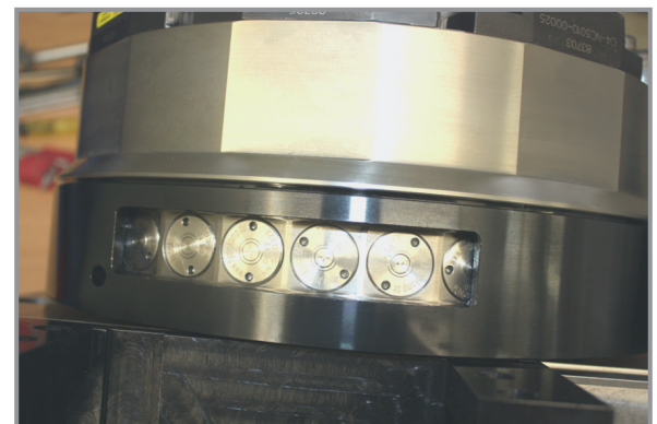
(2) Coupling nipples in the revolver fixture (with a total of 36 coupling nipples)
