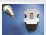
According to different cutting data, wire diameter, angle and workpiece thickness, the AccuteX controller automatically optimize parameters to maintain the best corner cutting performance with high accuracy, as well as cutting speed. Even on the small and continuous corners, accutex still can meet the best corner accuracy.
