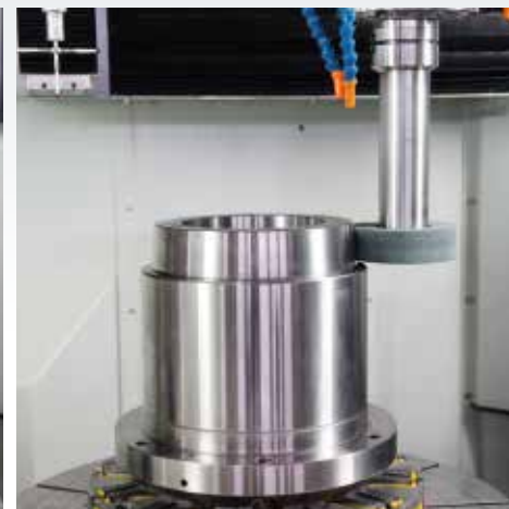
2-axes simultaneous OD cylindrical grinding (slop 5 degrees)
