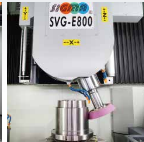
OD cylindrical grinding (grinding spindle at 22.5 degrees)
