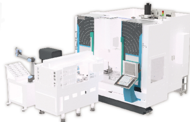
UB 660 Automated Production Line
