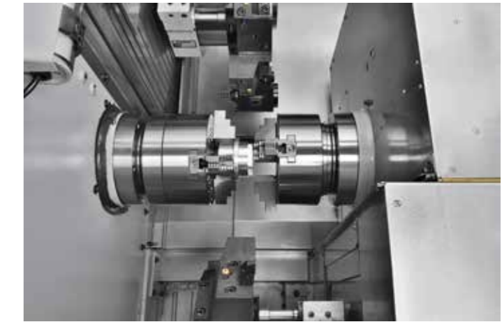
Synchronous parts interchange control
