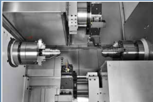
Opposite upper and lower turrets with a single Y-axis on the upper side
