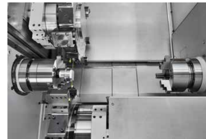
Twin path composite balance cutting control on SP1
