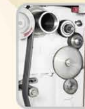
▲ Multiple threading system for cutting wormhas two-speed feed
