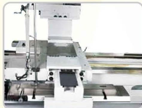
▲ Taper Turning Attachment +/- 7 degrees Travel 500mm (19.69")
