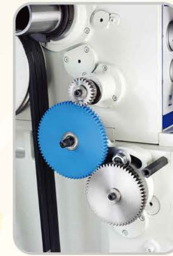
◀ Plastic gear on the rear side of headstock
