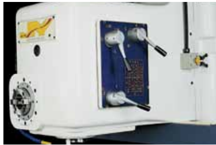
VERTICAL AND HORIZONTAL MILLING HEAD 立橫兩用銑頭
