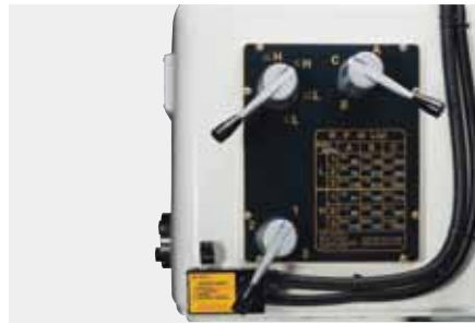
45-1500 RPM 18 SPEED CHANGE 45-1500 RPM 18段變速
