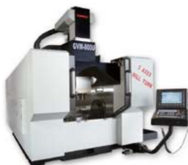
• GVM-800U 5 Axes gantry type machining center
