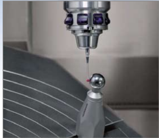
Inspecting and optimizing machine accuracy by calibrating rotary axes with kinematics
