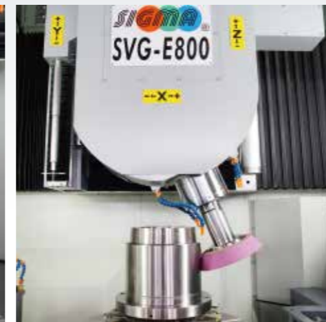
外徑平面研磨 (研磨主軸角度在22.5度時)
