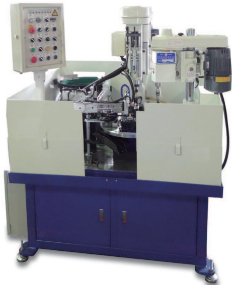
自動送料倒角、攻牙專用機 AUTO. FEEDING CHAMFER AND TAPPING SPECIAL PURPOSE MACHINE
