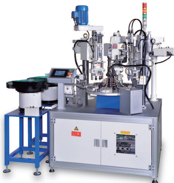
自動送料鑽孔、攻牙、鎖螺絲專用機 AUTO. FEEDING DRILLING / TAPPING / SCREW ASSEMBLY SPECIAL PURPOSE MACHINE
