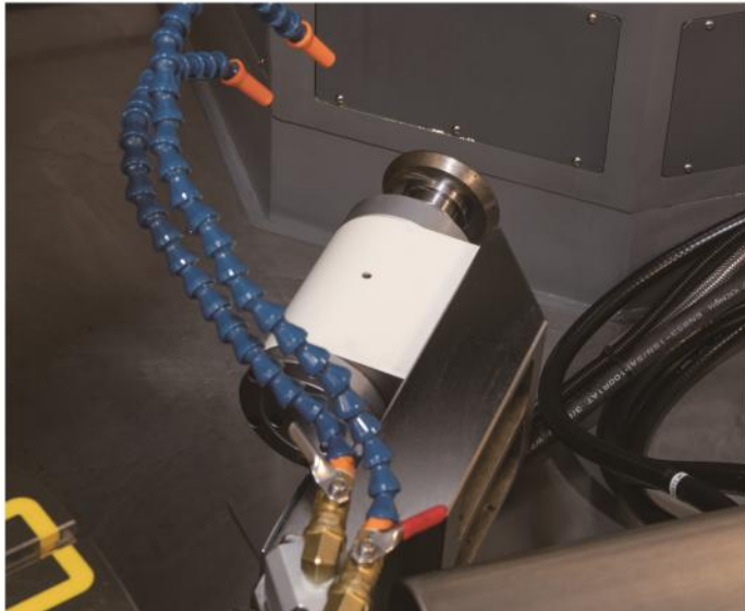
修砂器90度起降 90 degree rotation dresser
