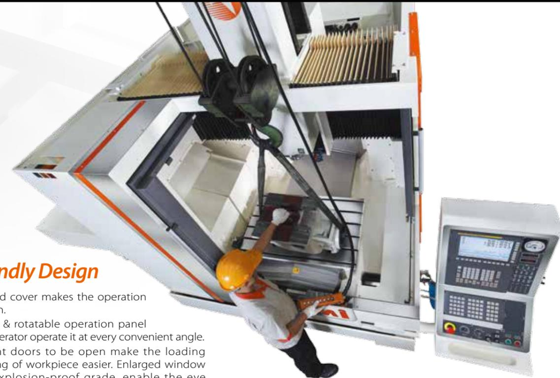
*H6 new two adjacent doors to be open make the loading and unloading of workpiece easier.*
