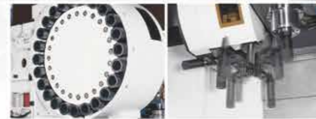
24T, BT40, ARM type ATC (Standard)
