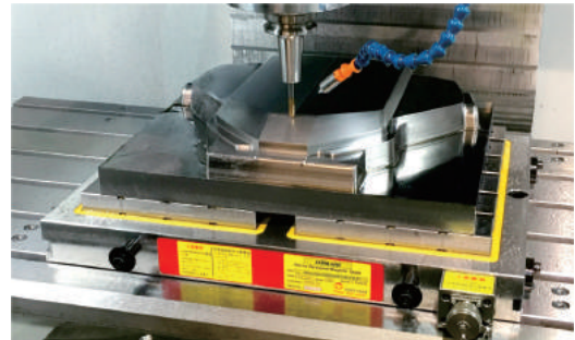
EPPM-B Series Flux Line 25 mm, Pole Size 50x50 mm Magnetic force: 1250 ±5% Kg/4 poles
