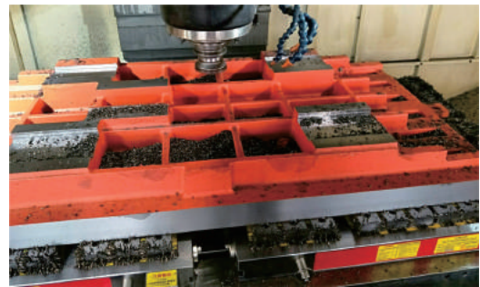
EPPM-D Series Flux Line 40 mm, Pole Size 70x70 mm Magnetic force: 2800 ±5% Kg/4 poles
