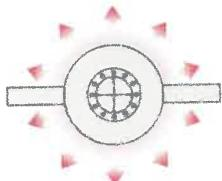
The center of the axis is maintained, even if the frame of the spindle expands.
